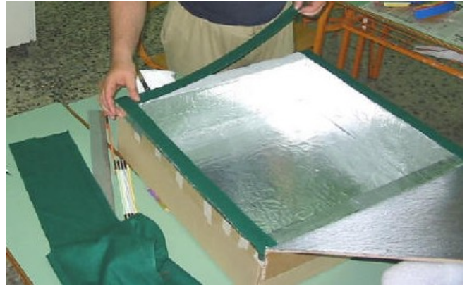
Photo 8: Sticking some pieces of felt on the top frame of the box cooker, so the glass rests firmly ...
