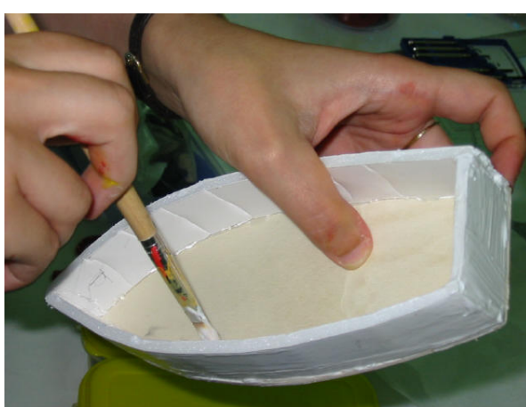
Photo 1: Pieces of paper foam board have been glued around the basis of the boat hull made out of balsa wood. Some extra white glue is added from the inner part of the construction for better fixing.
