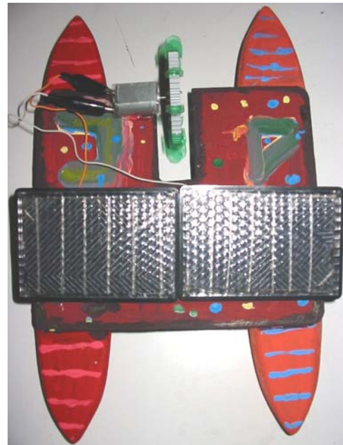
Photo d: This is an idea of a solar river boat with two floaters out of Styrofoam and a deck of thin plywood. The interesting piece in this construction is the water wheel made out of a big gear with plastic fins attached to it, cut out of a plastic soda bottle.
