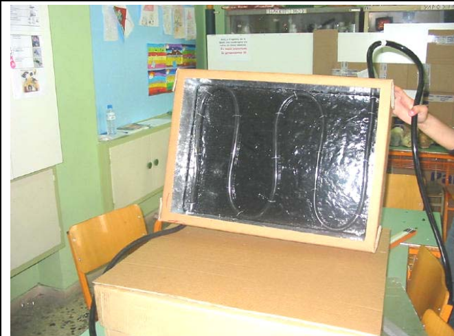
Photo 3: Tying the tube in its place, forming a serpentine or continuous "S" arrangement ...
