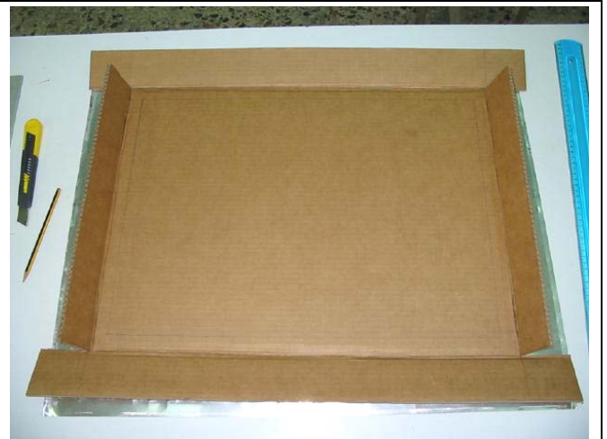
Photo 4: Cutting out a piece of corrugated paper to form the top lid of the solar collector ...
