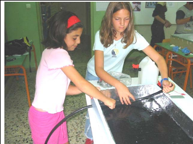
Photo 1: Inserting the black plastic tube inside the collector box made out of polystyrene ...
