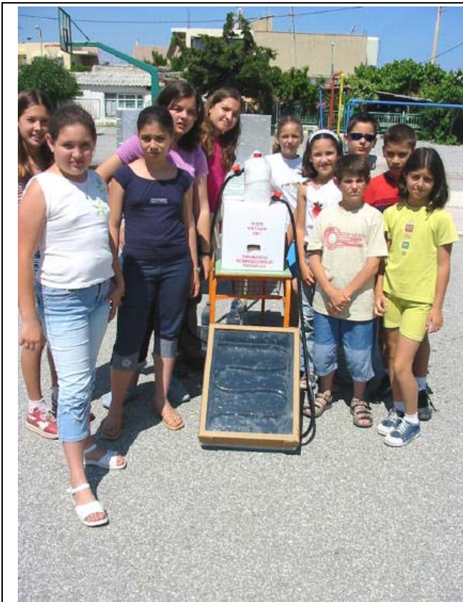
Photo 7: The testing of a “serpentine solar heater” constructed with flexible black tube, inside a collector box and a plastic can used as a water tank.
