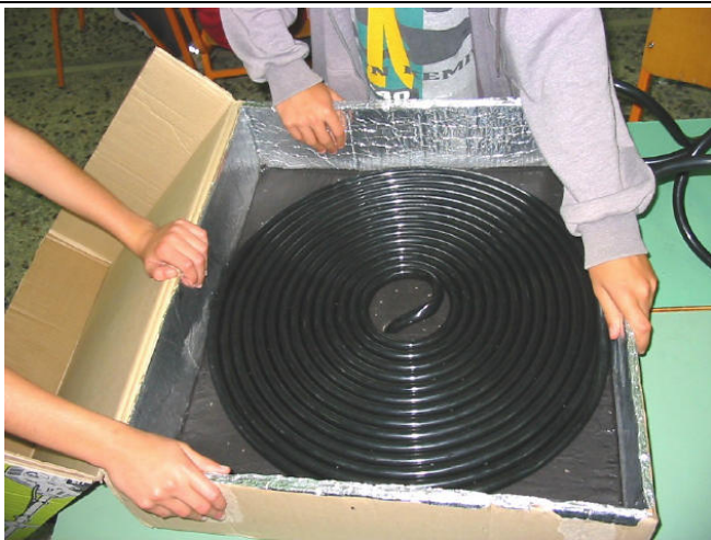
Photo 3: The spiral tube is now in place inside the cardboard box and needs to be tied ...
