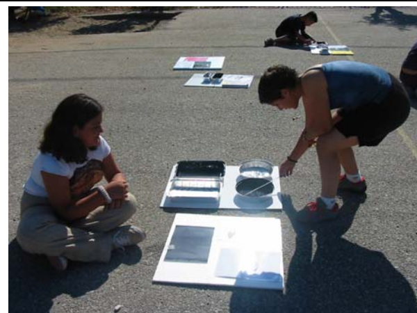
Photo 3: Another pair of children experimenting with different settings of aluminium containers. Notice the Styrofoam frames under the aluminium containers, providing insulation with the ground.
