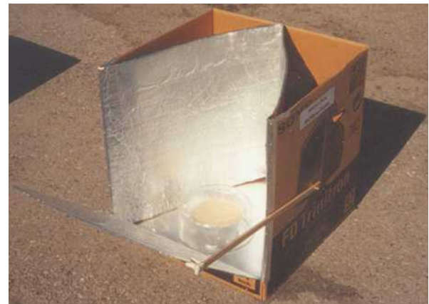
Photo 6: Another "reflective open box" solar cooker presented in a school science fair. Notice the piece of wood used as a prop to hold and adjust the front reflector.
