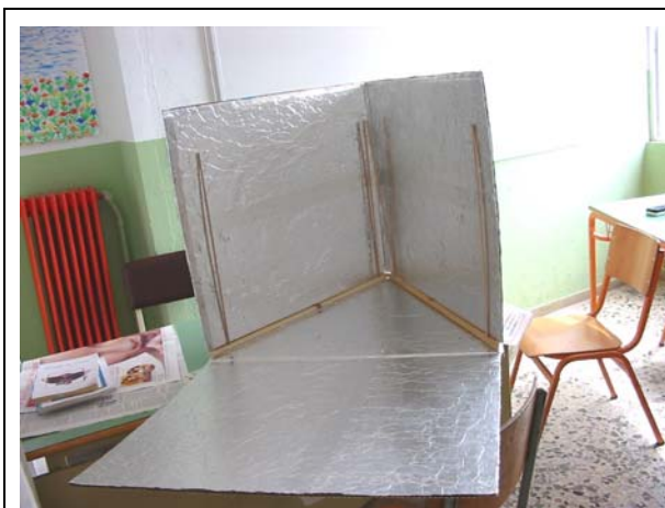
Photo 1: Constructing in class a portable open panel solar cooker with two pieces of cardboard. Notice the two pieces of board with the two pairs of round wooden sticks supporting the "V" shaped reflectors ( front view ).
