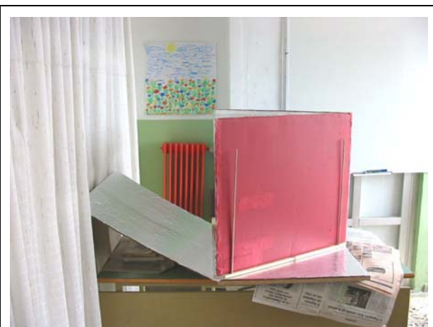
Photo 2: Constructing in class a portable open panel solar cooker with two pieces of cardboard. Notice the two pieces of board with the two pairs of round wooden sticks supporting the "V" shaped reflectors ( side view ).
