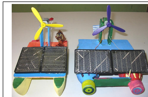
Photo 11: Two solar catamaran boats. Their floaters are made out of expanded polystyrene (left) or used plastic bottles (right) and they both moved with a helix.
