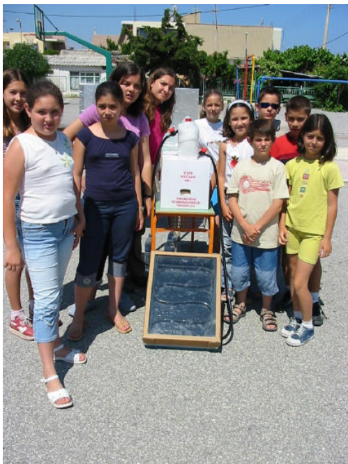
Photo 3: The testing of a “serpentine solar heater” constructed with flexible black tube, inside a collector box and a plastic can used as a water tank.
