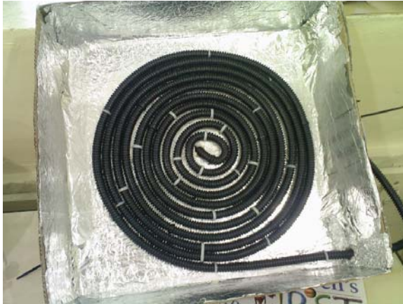
Photo 15: The tube arrangement of a spiral solar water heater (Stella Maris College Junior School, MT).
