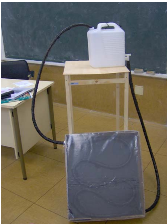
Photos 16: A serpentine solar water heater with its tank (Colegio de Educación Infantil e Primaria Froebel, ES).
