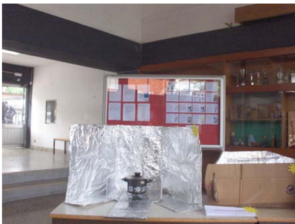
Photo 17: An open panel solar cooker at an exhibition (Escola Antré Soares, PT).
