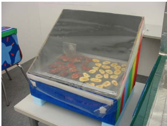
Photo 10: A “solar dehydrator” (Sun dryer) out of a cardboard box, for drying out fruits and vegetables (9 th Primary School of Rethymno, Crete, EL).
