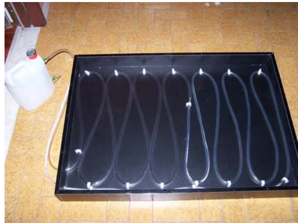
Photos 2 & 3: The preparation and construction of a serpentine solar water heater (Scuola Secondaria di 1 o Grado C.B. Cavour, IT).
