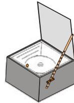
**2** You may insulate the bottom of the *inner box* in the same way and then put it inside the outer box. It is better to choose boxes that fit one inside the other, reaching roughly the same height, leaving an empty space of 3-6 cm wide, in every side all around.
