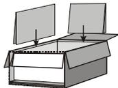
**5** Take each flap of the outer box, fold it along the continuous lines and cut it along the dotted lines. Notice that flaps *b* & *d* are treated differently from flaps *a* & *c* (see drawing).
