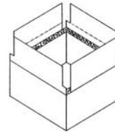
**7** Glue the dull side of aluminium foil all around the sides of the inner box. The base of the solar box cooker is now ready.
