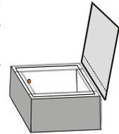
**9** A glass frame needs to be cut in a shape to fit the open top of the base. The glass frame is safer and has greater endurance if its sharp edges are buffed. You may glue pieces of felt along the top edges of the box to provide a smooth, firm resting place for the glass frame and to seal in the heat. Optionally, a wooden knob can be fixed on the glass. The solar box cooker is now ready to cook!
