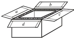
**6** After cutting along the dotted lines, the four flaps are shaped as shown in the drawing. Fold each flap over the insulated area and glue it inside the inner box. If the flap comes a bit short and does not cover the whole side, you may glue extra pieces of cardboard to cover that area.
